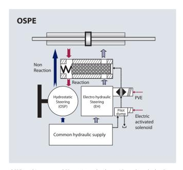
${\it OSPE combines proven OSP steering technology with an electrohydraulic steering valve.}$
