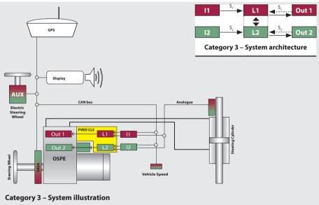
The safety function architecture is the minimum architecture required to meet the result of the hazard and risk analysis.
