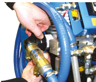
FA 016 with screwed-in suction strainer set FA 016.1775
