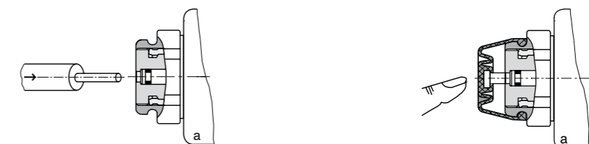
Basic versions of the manual override using pin or push button placed in the protective rubber sleeve.
