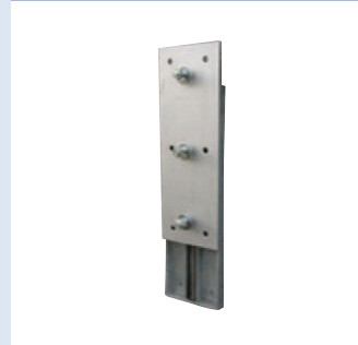
Back plate for 750 mm buffer 965 x 250 x 66 mm Weight: 47 kg Spring loaded. Follows the truck when loading.
