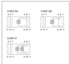
CHM7 PILOT OPERATED CHECK VALVE SERIES 11
