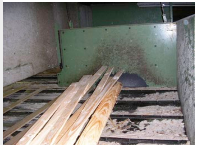
Impact protection for wooden battens
