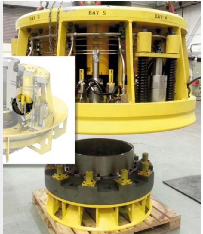
MAGNUMS allow for emergency quick disconnection of the pipelines from the oil rigs Subsea Technologies Ltd, Aberdeen, AB12 3AY, UK
