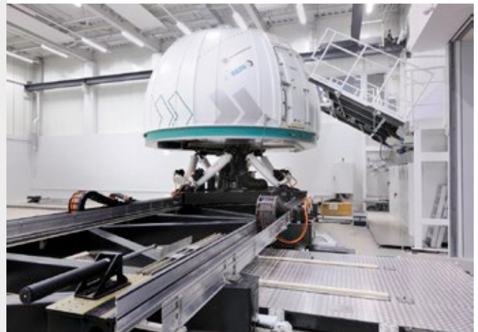
ACE safety shock absorbers protect end positions in two axes of a driving simulator Bosch Rexroth BV, Boxel 5281 RV, The Netherlands and University of Stuttgart - FKFS, 70569 Stuttgart, Germany
