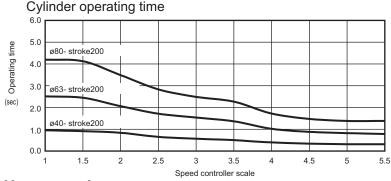
Conditions SCA2, no load, vertical, piping tube ø6-1m 0.5MPa
