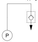
Reverse flow prevention of 2 fluid control Prevents reverse flow of multiple pressures and multiple fluids in merged circuits
