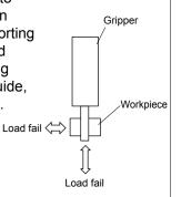
Mounting the attachment When mounting the attachment to the finger, to prevent any effect on the gripper, support with a wrench, etc., when tightening so that the finger is not twisted.
