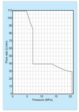
\* Operating flow rate at the maximum pressure in continuous operation: 16 L/min maximum
