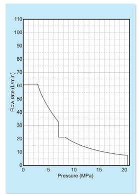
\* Operating flow rate at the maximum pressure in continuous operation: 6.5 L/min maximum
