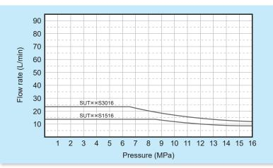
\* Operating flow rate at the maximum pressure in continuous operation: SUT\*\*S1516: 5 L/min maximum SUT\*\*S3016: 5 L/min maximum
