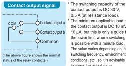
contact output is DC 30 V, 0.5 A (at resistance load). The minimum applicable load of the contact output is DC 10 mV, 10  $\mu\text{A},$  but this is only a guide to
