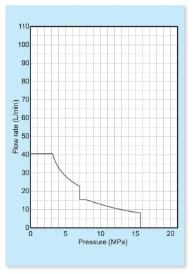
$^{\ast}$  Operating flow rate at the maximum pressure in continuous operation: 8 L/min maximum
