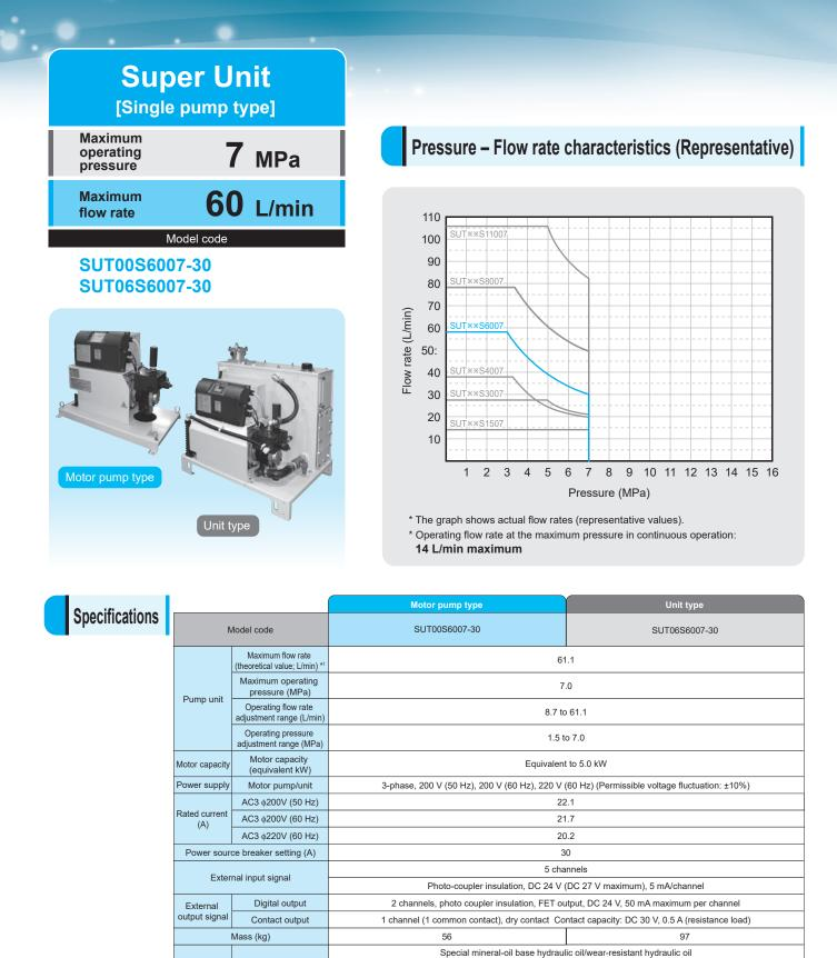
Tank capacity (L) 60 Standard coating color Ivory white (Munsell code 5Y7.5/1) The pump flow rate has been factory-set to the maximum discharge rate. The maximum discharge rate given in the table above is a theoretical value, not a guaranteed value Consult Daikin about the use of hydraulic oils other than mineral-oil base type (e.g. hydrous/synthetic) such as water-glycol hydraulic oil. Note) \*1:
