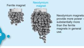
\*1: A compound of neodymium (Nd, rare-earth element), iron (Fe), and boron (B). Neodymium magnets are known to have superior magnetic properties.
