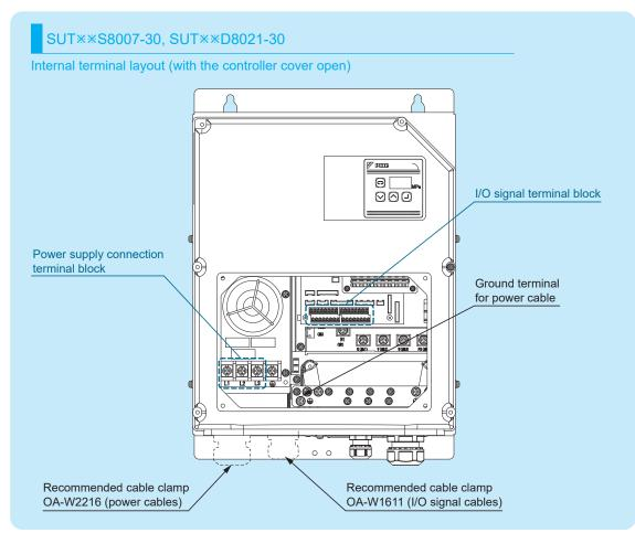
\* Main power supply connections: Connect a 3-phase AC power supply (200 V/50 Hz, 200 V/60 Hz, or 220 V/60 Hz) to the power supply terminals (L1, L2 and L3), and connect a ground cable to the ground terminal.
