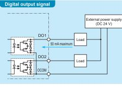
\* The digital output common terminal can be either positive or negative. \* Prepare an external power supply (DC 24 V ± 1 V, 0.5 A or more). \* The maximum output current of the output circuit is 50 mA per channel.
