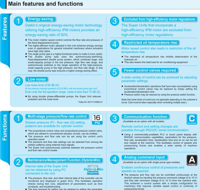
The time required for setting can be slashed by editing the parameter settings on the PC and writing them to the unit in a batch. The ability to read and save settings facilitates management.
