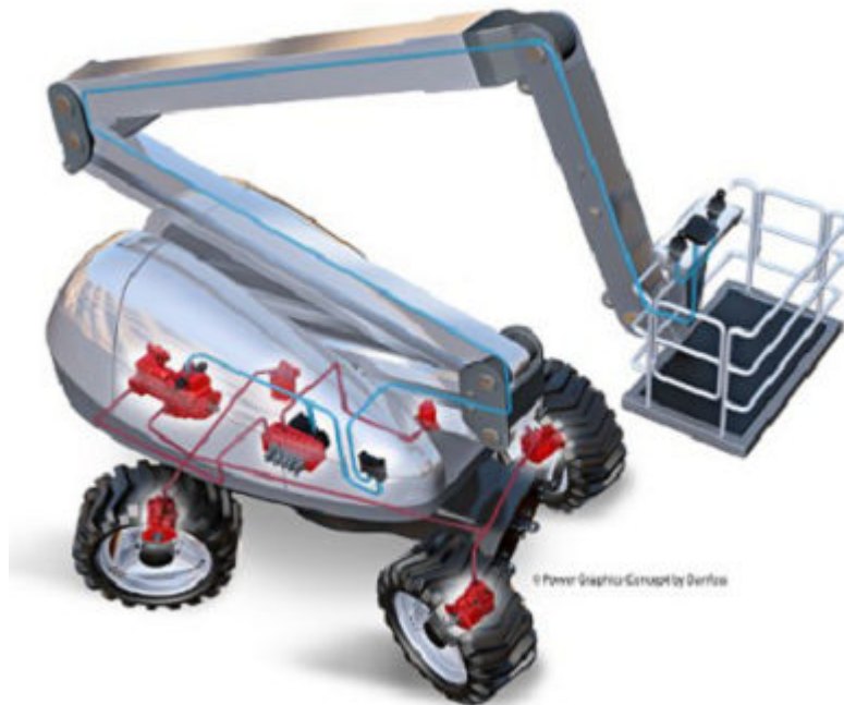
Example of a control system for man-lift
