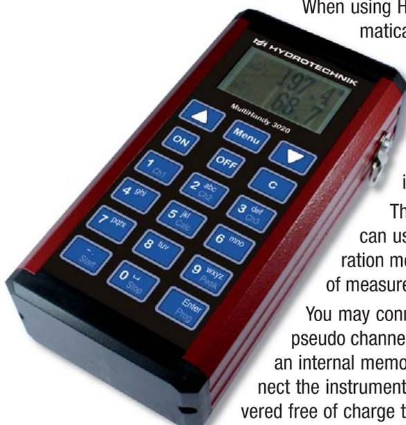
When using HySense® sensors with ISDS signal, the measuring instrument automatically detects the connected sensors during boot-up and takes over all parameters: measuring range, physical measurand, units, output signal and characteristic curve (linearisation). Mixed-up sensors are avoided, the manual input of numerous data is superfluous.
