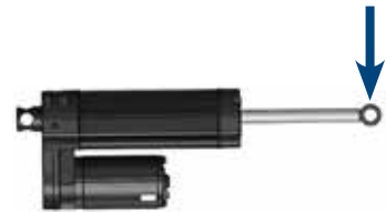
Figure 8 Radial load also side loading
