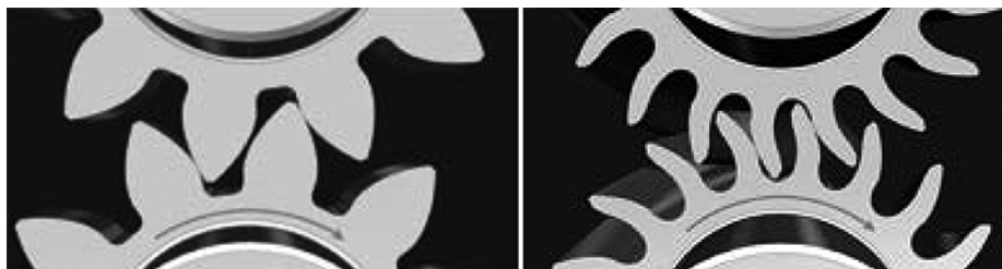
Standard gear pump (11-teeth) versus shhark® (19-teeth) technology
